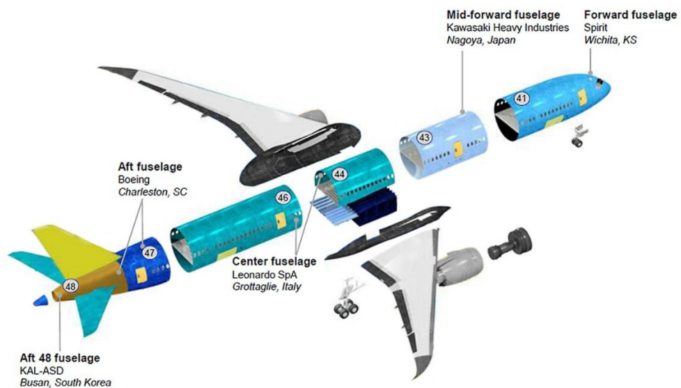
Figure 5. Boeing Suppliers Used To Produce 787 Fuselage Sections
